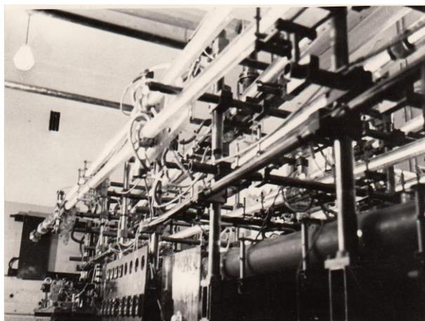
**Fig. 2.** “Zig-Zag”- CO<sub>2</sub>-laser created by A.I. Barchukov FIAN 1970 [2].
